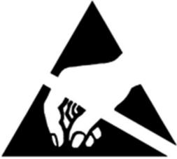
The ESD susceptibility symbol incorporates a reaching hand in a triangle with a slash through it and is used to indicate that an electrical or electronic device or assembly is susceptible to damage from an ESD event. Used to identify ESDS [ESD sensitive items] and that personnel should be grounding when unpackaging or handling that item. It is also referred to as the ESD sensitivity symbol or ESD warning symbol.
