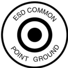
This symbol is established to indicate an ESD common point ground, which is defined by ANSI/ESD-S6.1 as "a grounded device where two or more conductors are bonded."
