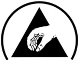
The ESD protective symbol differs from the ESD susceptibility symbol, by the addition of an arc around the outside of the triangle and the omission of the slash across the hand and the triangle.
